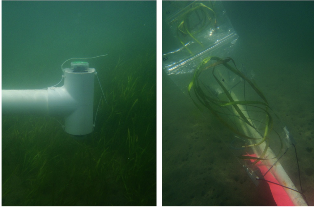
Figure 4. Deployment of autonomous light and T sensors (left). Detail of transparent incubation chamber (right).
